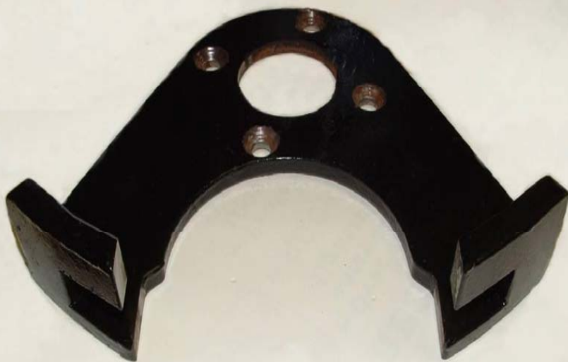
Backing plate for Toro / Eldorado type calipers, fork design similar to drop forged front knuckle
